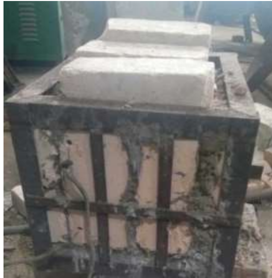
Figure 3: Fabricated 4 kg Electric Furnace With Cover
